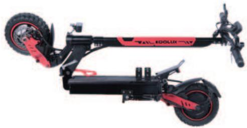
2. First, release the silver secondary lock on the side, straighten the steering column, then lift the folding lever and press it firmly into the groove until it clicks into the locked position.
