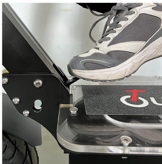
② Loosen the pole, pulling the lock backward, and fold the pole down.
