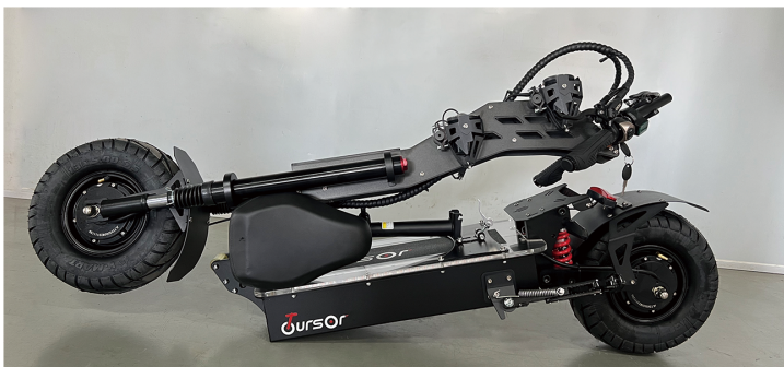
② Hold the handlebar, press the folding lock with your feet and fold it
