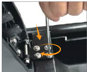
Install the seat cushion and tighten the four screws
