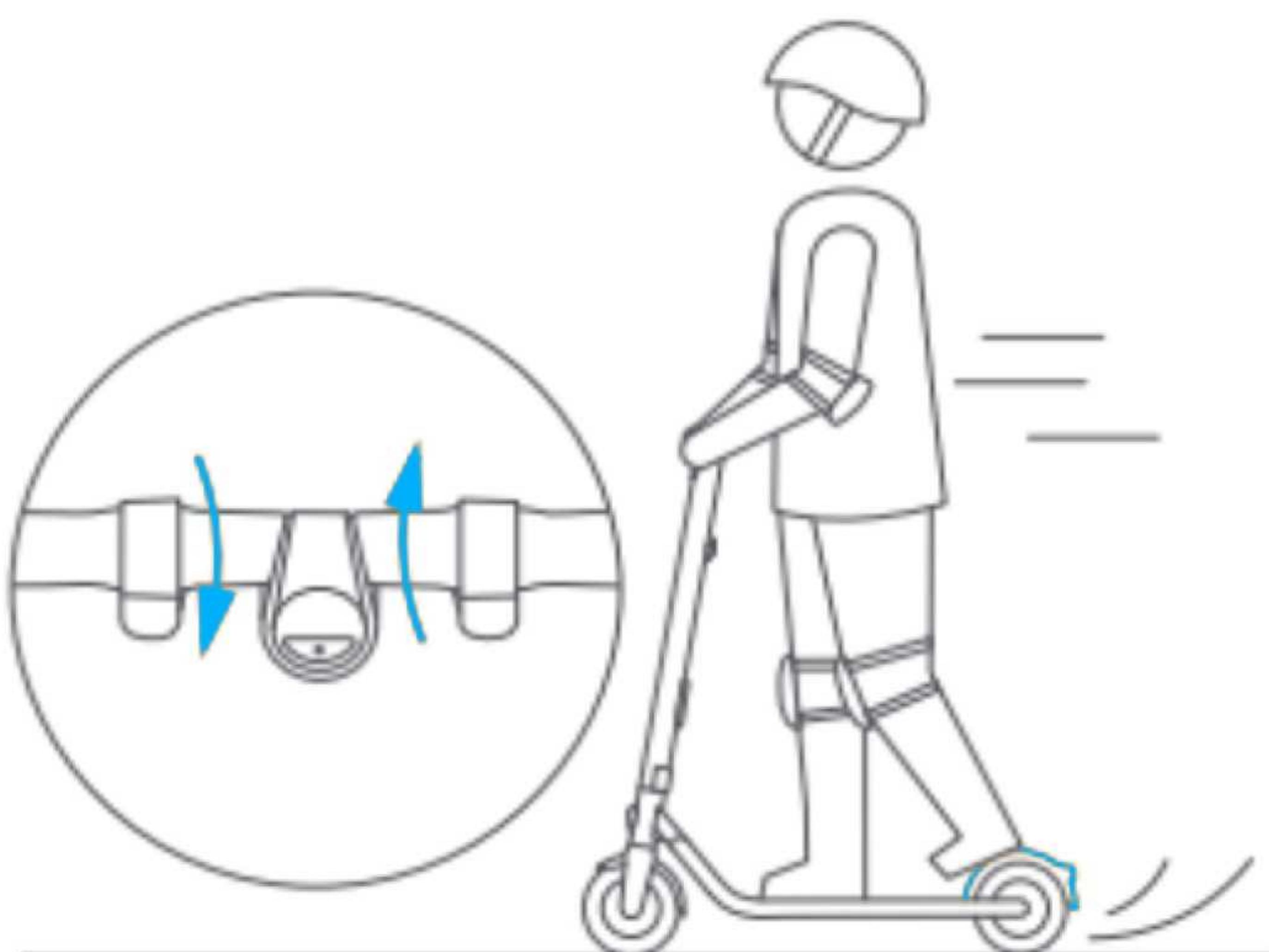
5. Slow down by releasing the throttle. Squeeze the brake and stamp the rear fender with your foot at the same time for a brake.
