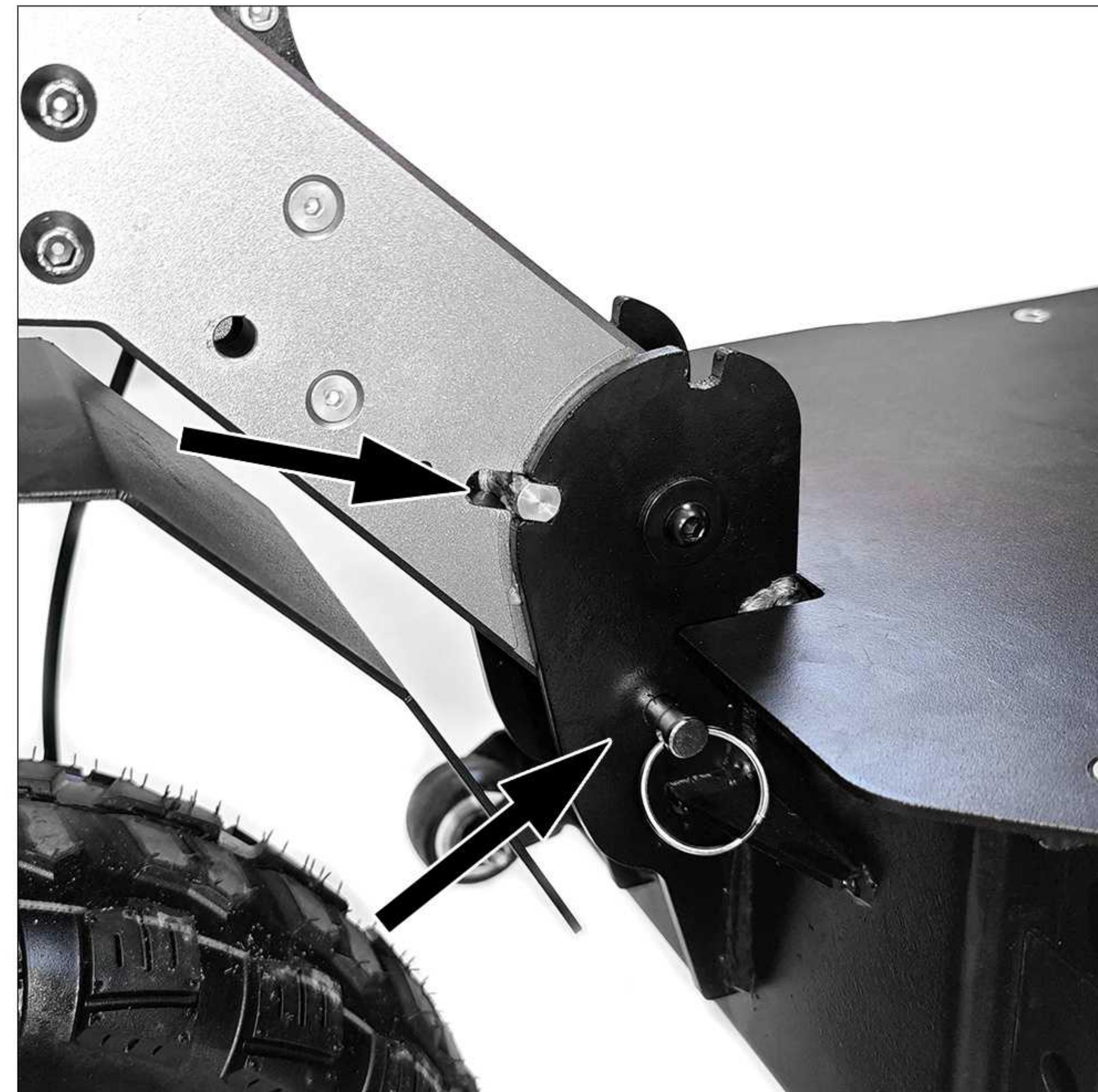
3. Install the stem and tighten the screw at the top.
