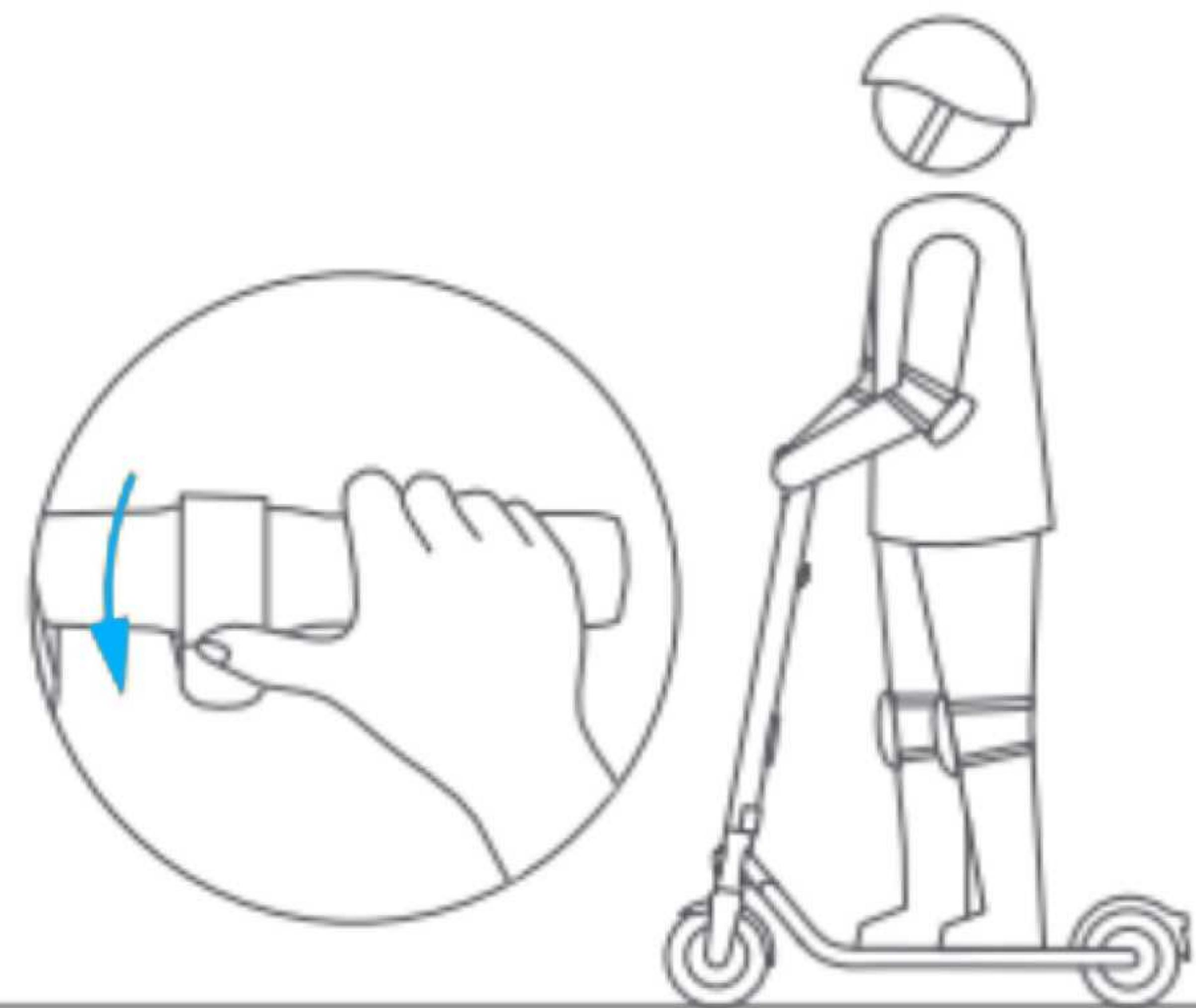
4. Put your other foot on the foot deck to keep both feet stable. Press the throttle to speed up when you are balanced.
