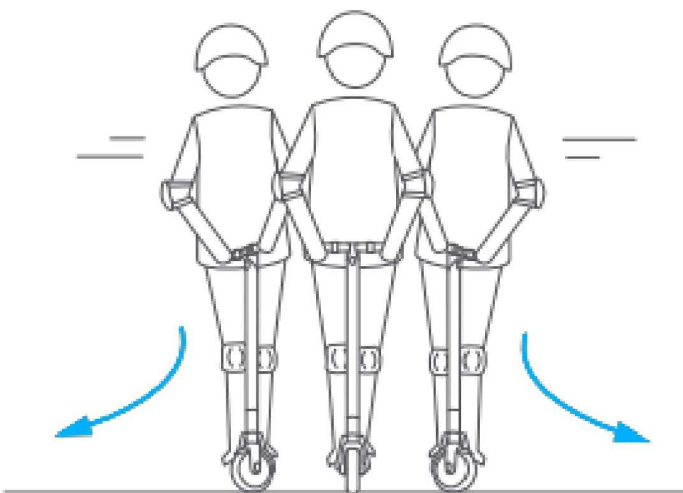
⚠️ DO NOT rotate the handlebar violently while driving at high speed.
