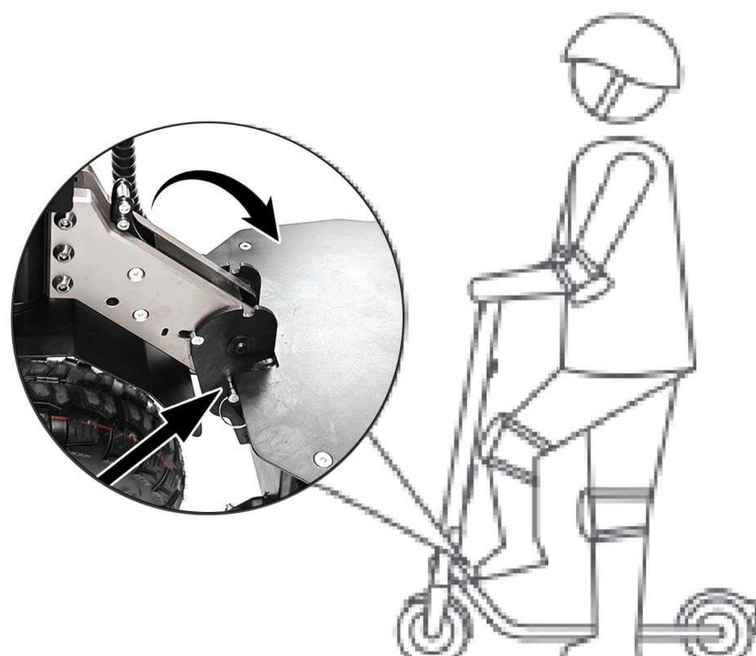
Make sure that the scooter's turned off. To fold, unlock the folding mechanism. Then fold the handlebar down.
