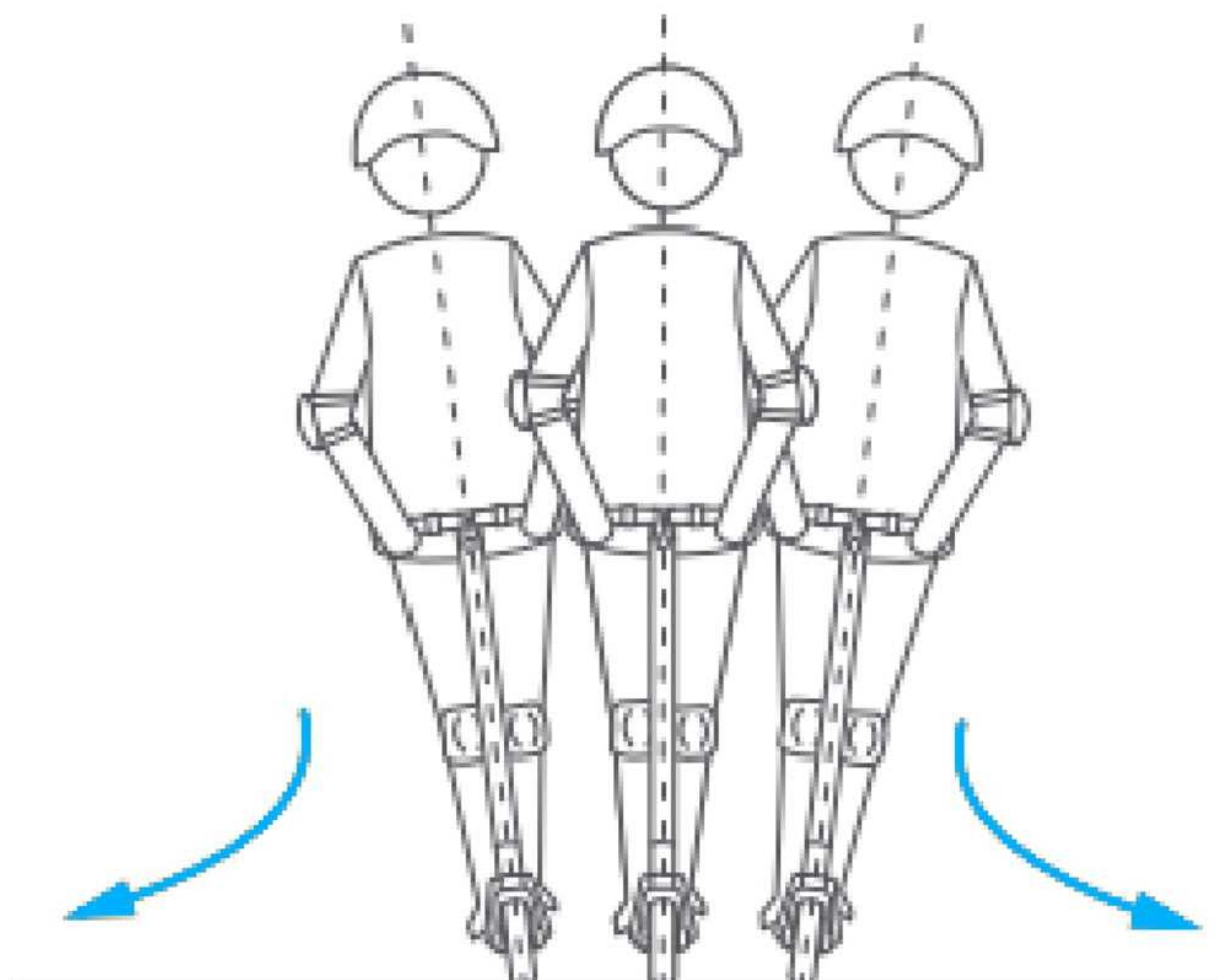
6. To turn, shift your body and turn the handlebar slightly.
