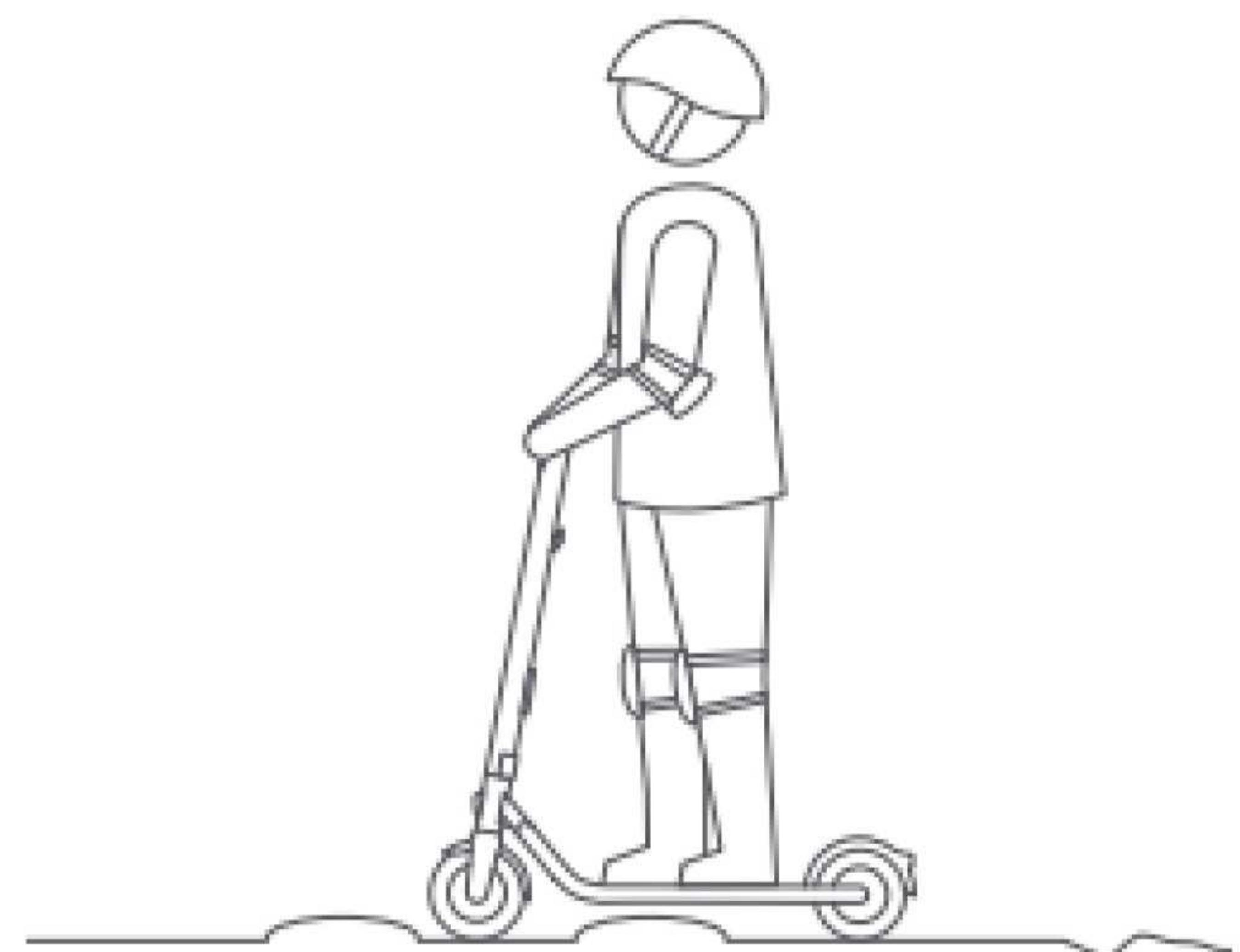
⚠ Keep your speed between 3.1–6.2 mph (5–10 km/h) when you ride through speed bumps, elevator door stills, bumpy roads, or other uneven surfaces. Slightly bend your knee to better adjust mentioned surfaces.
