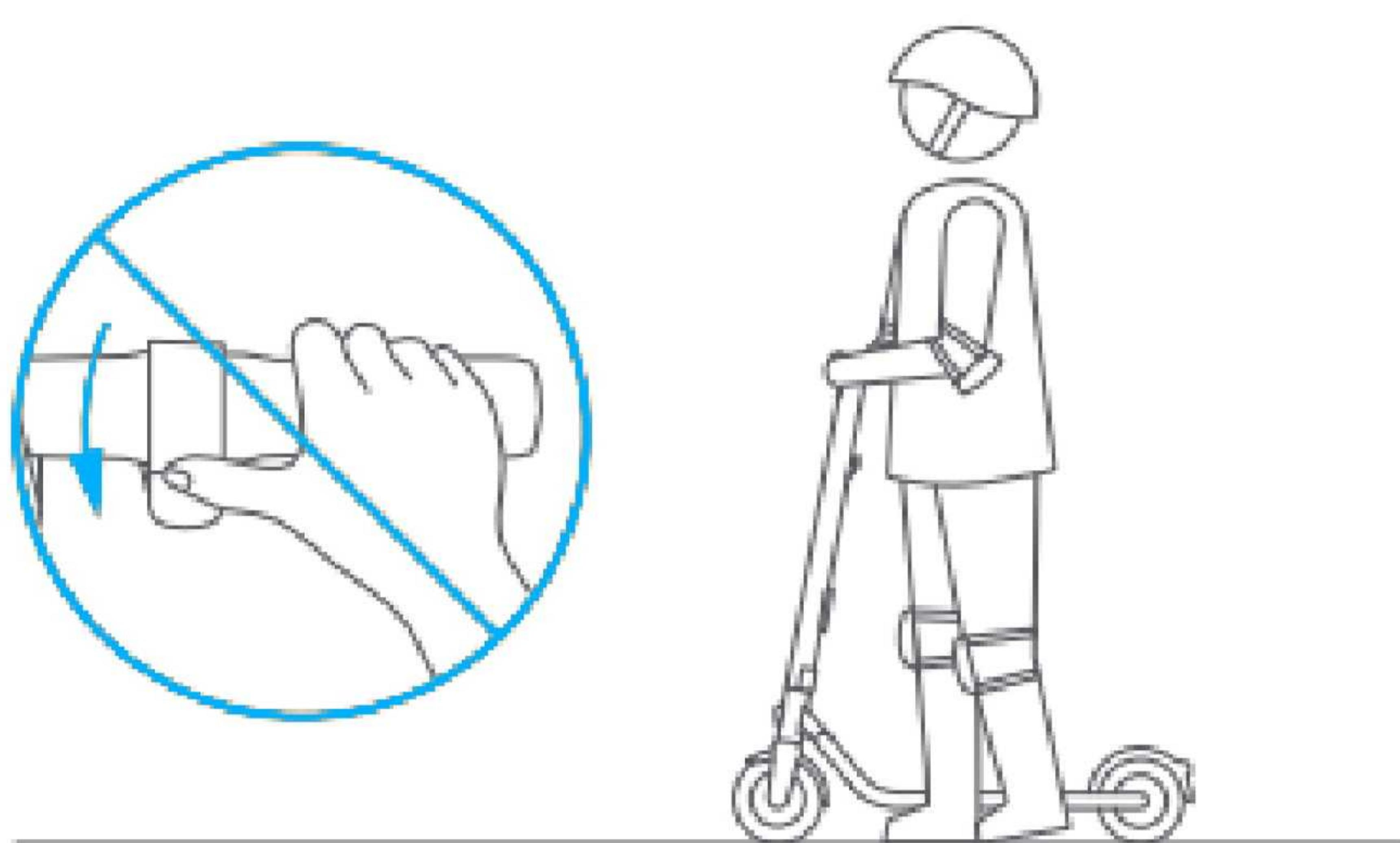
⚠ DO NOT press the throttle when walking with the scooter.
