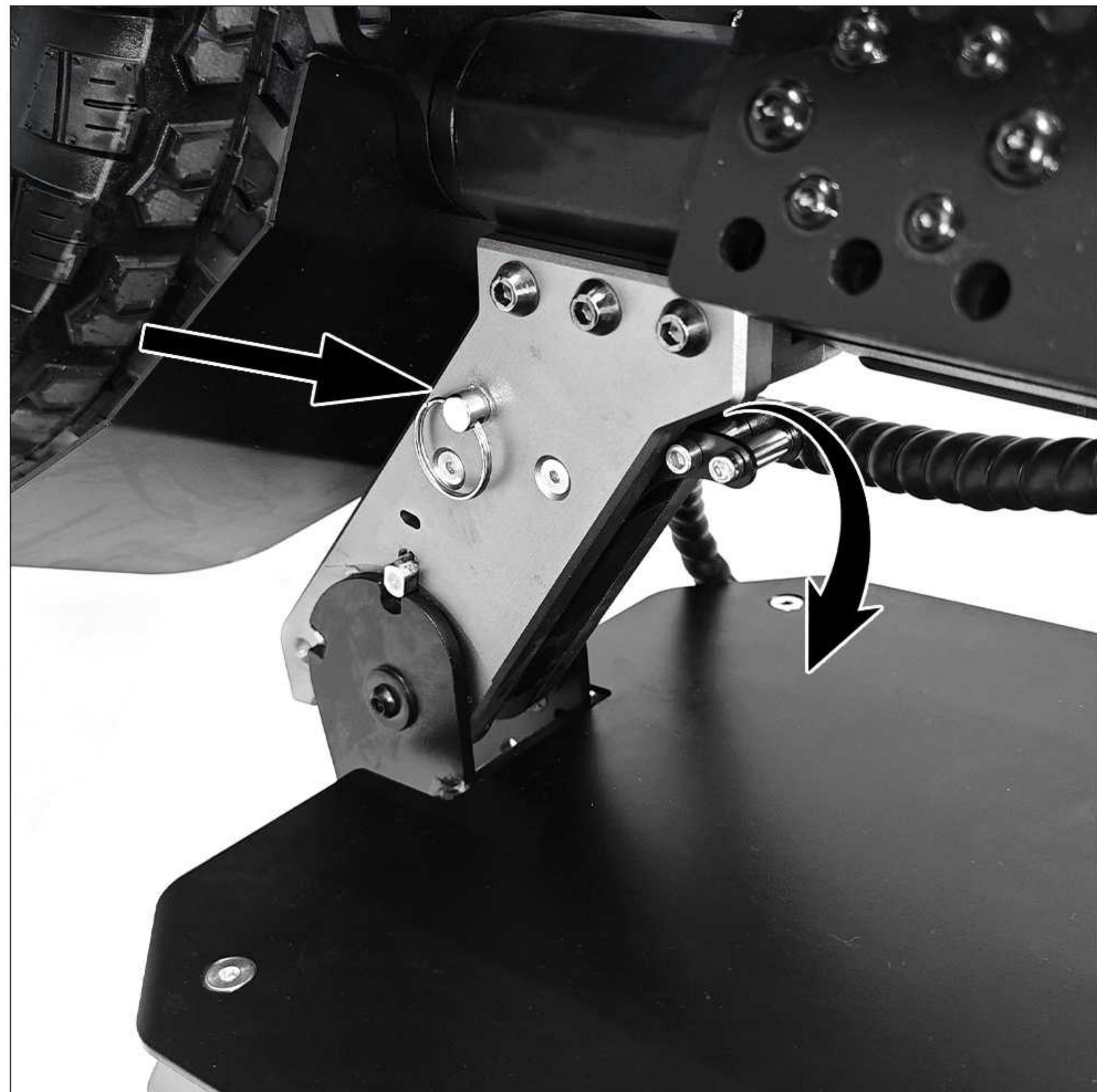
2. After unfolding the frame, the metal column at the fold will move to the front position. Then, insert the metal safety pin into the hole below.
