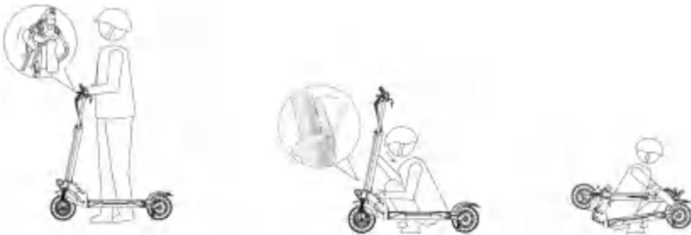
The scooter needs to be turned off before folding. Pull out the lock, then grab the pole and pull down to fold.
