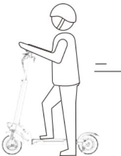
2. Step on the deck with one foot, and slowly kicks off the other on the ground. When the scooter starts to coast, put both feet on the deck and press the accelerator (the accelerator initiates once the coasting speed exceeds 5km/h).
