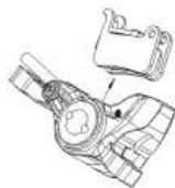
Figure 2-5 Removing/Assembling the Brake Pads and Accessories
