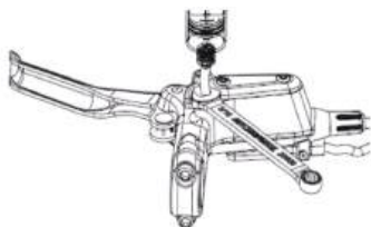
Figure 5-3: 8mm open end spanner to loosen/tighten the main body of the caliper into the nozzle screws.
